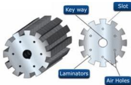
Figure 3: Armature of DC machine
